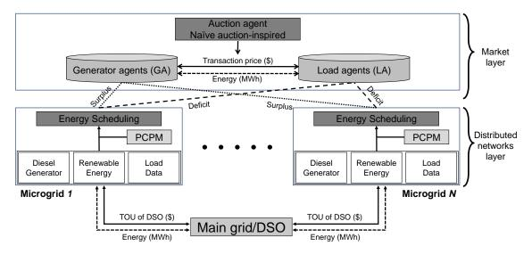
**Figure 1.** The overall structure of multiple microgrids. PCPM: predictor corrector proximal multiplier; TOU: time of use; and DSO: distribution system operator.
