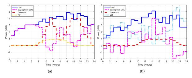
**Figure 5.** Load profile and power scheduling based on OPF operation: (**a**) microgrid 1; and (**b**) microgrid 2.
