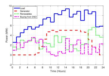
Figure 8. Load profile and power scheduling based on the centralized optimal power flow.
