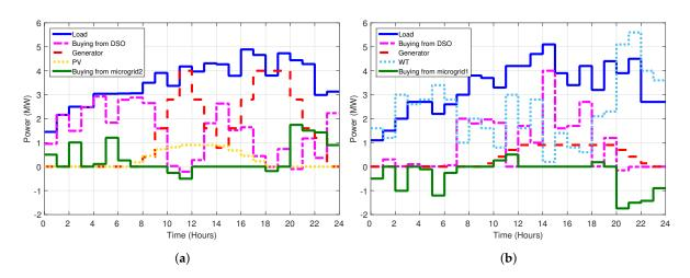
**Figure 7.** Case 3: load profile and power scheduling based on the transaction-enabled OPF algorithm. (a) Microgrid 1; and (b) microgrid 2.
