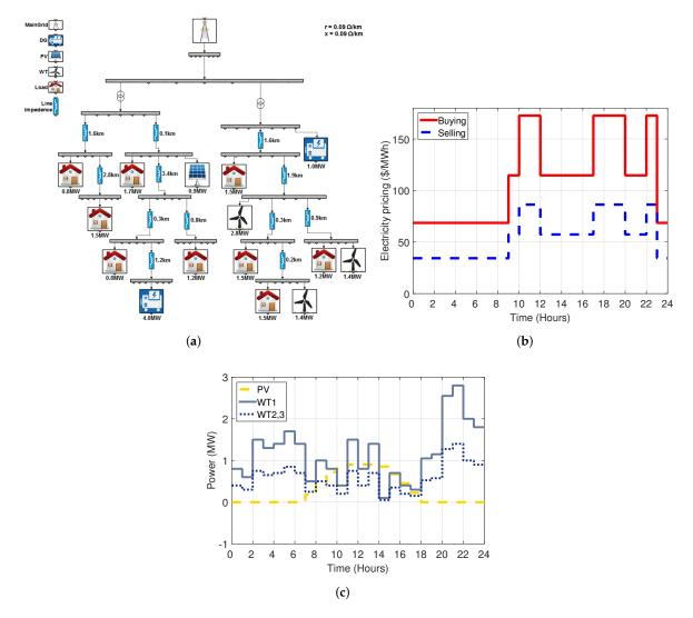
**Figure 3.** (**a**) The topology of microgrids; (**b**) transaction price from the main grid; and (**c**) renewable energy profile.
