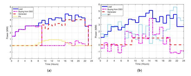
**Figure 4.** Case 1: load profile and power scheduling based on non-OPF operation. (**a**) Microgrid 1; and (**b**) microgrid 2. OPF: optimal power flow.
