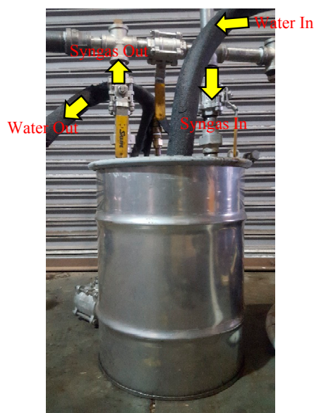
Figure 6. Oil bubbler unit for treatment III.
