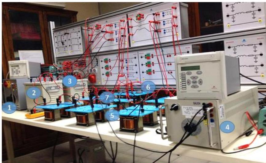
**Figure 13.** Laboratory setup for  $2 \times 25$  kV power system fault location testing.
