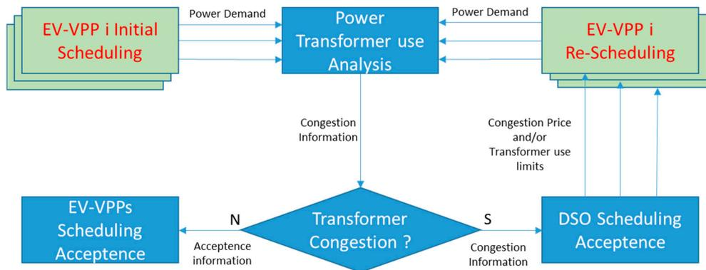
**Figure 2.** Flowchart of HV/MV power transformer congestion management.
