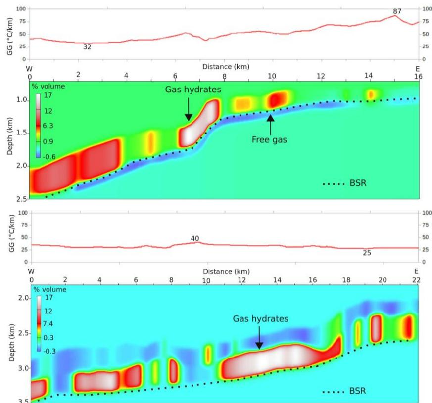
**Figure 3.** Gas hydrate (positive values) and free gas (negative values) concentration models. The BSR is indicated by dotted lines. GG (red lines) indicates the geothermal gradient estimated by BSR depth. See text for details. The numbers reported across the red line indicate the upper and lower GG values.
