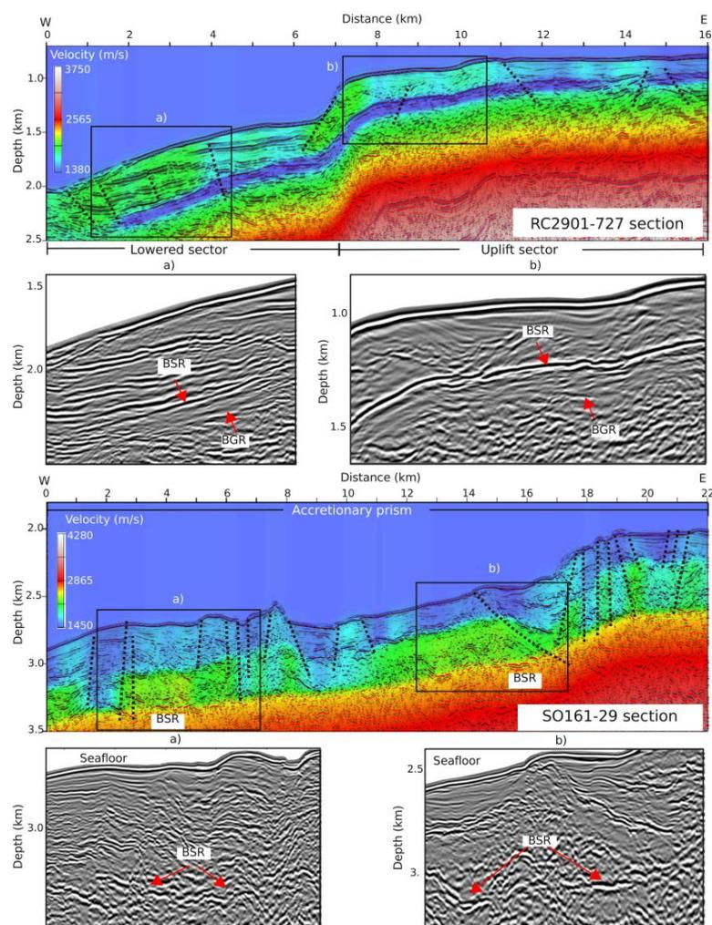
**Figure 2.** Velocity model superimposed to the Kirchhoff pre-stack depth migration (PreSDM) sections of the northern (**upper** panel) and southern (**lower** panel) sectors. The rectangles in the sections indicate the position of the zooms (a and b), in which the bottom simulating reflector (BSR) and the free gas reflector (BGR) (if present) are indicated by red arrows. Faults and fractures are indicated by dotted lines.
