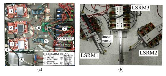
**Figure 8.** Experimental setup: (a) control platforms and drivers; and (b) LSRMs.
