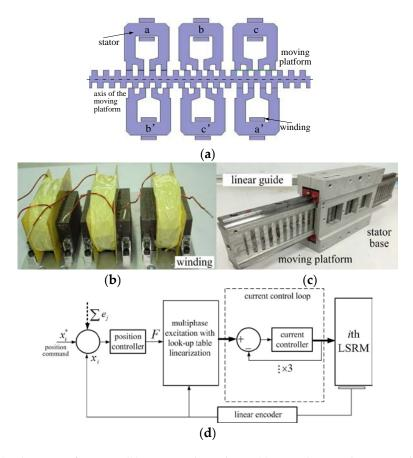
**Figure 6.** (a) Schematic of LSRMs; (b) stator and windings; (c) stator base and moving platform; and (d) LSRM control diagram.
