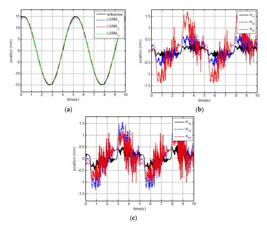
**Figure 9.** Tracking profiles: **(a)** LSRMs; **(b)** error to reference; and **(c)** relative error response with consensus algorithm only.
