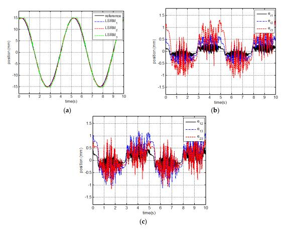
**Figure 10.** Tracking profiles: (a) LSRMs; (b) error to reference; and (c) relative error response under leader–follower–observer feedback with IMC.
