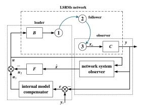
Figure 3. Control diagram of LSRM network.
