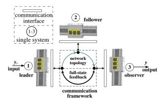
Figure 7. Hardware construction of LSRM network.
