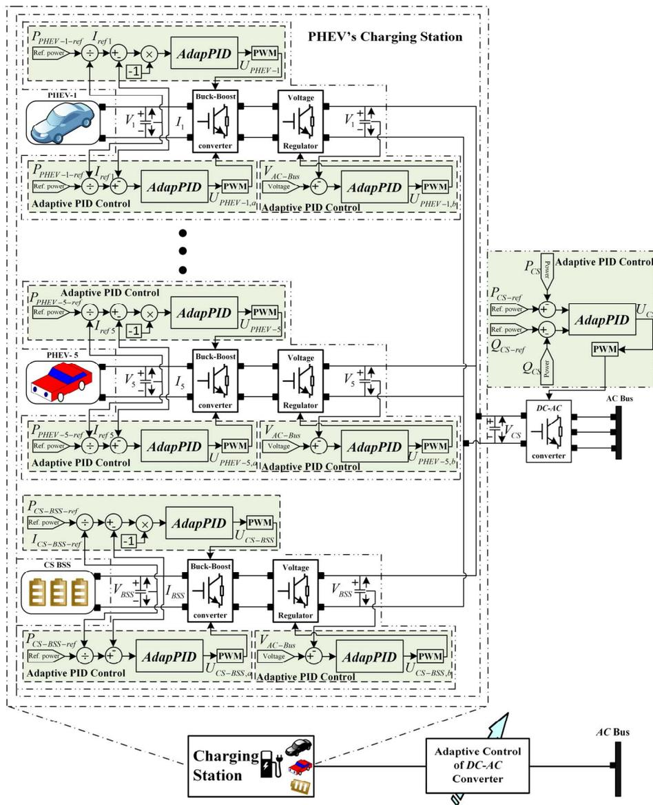
Figure 1. PHEVs charging station.
