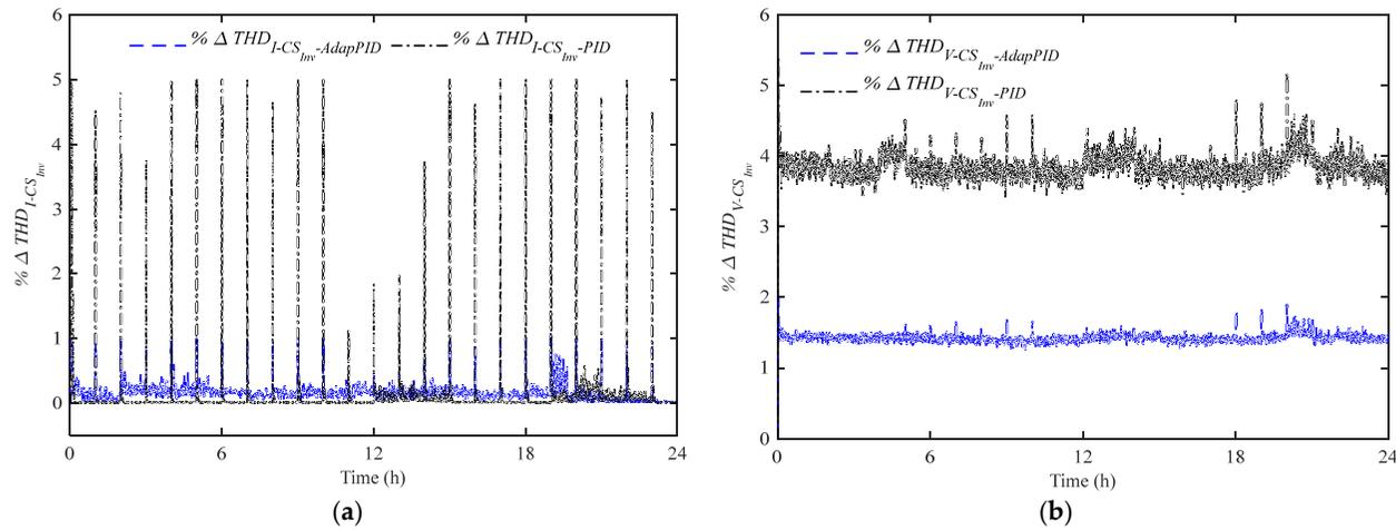
Figure 8. % change in CS converter (a) Current THDs (b) Voltage THDs.
