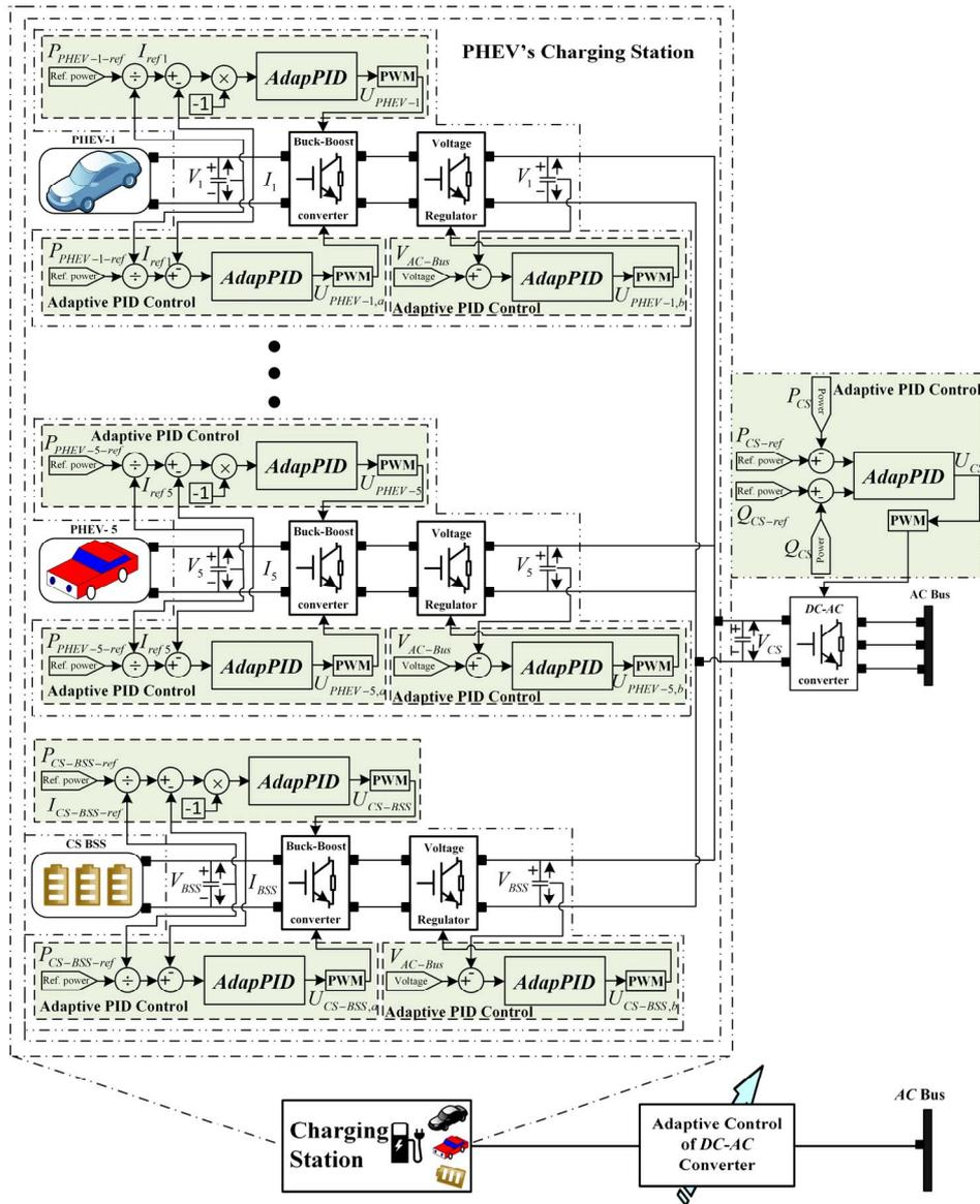
Figure 1. PHEVs charging station.
