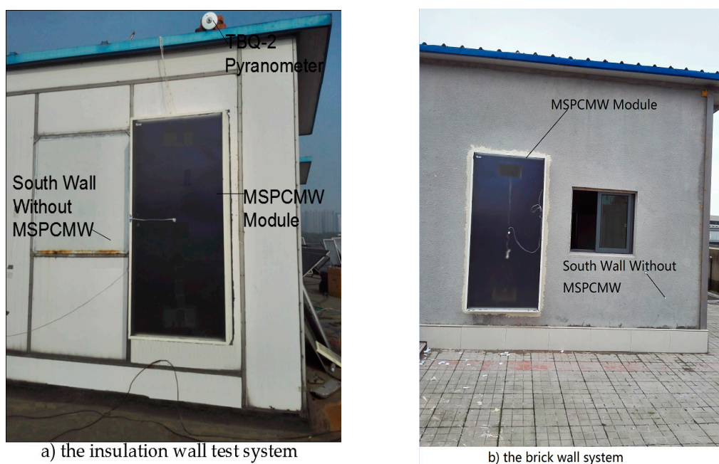
Figure 2. Exterior view of the two test systems: (a) the insulation wall test system and (b) the brick wall test system.
