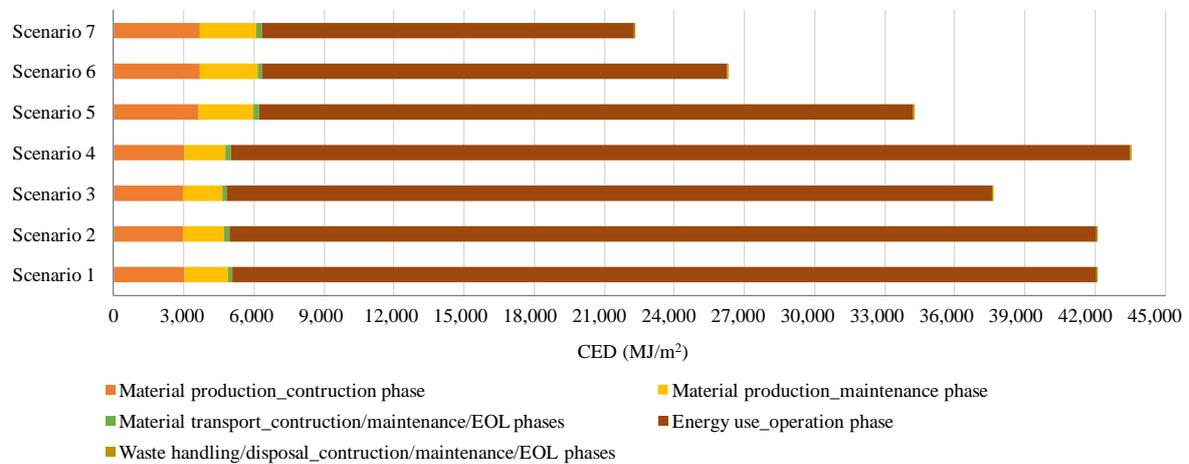
**Figure 4.** Cumulative energy demand results normalized by the floor area and referred to 50 years of building life span after the renovation.
