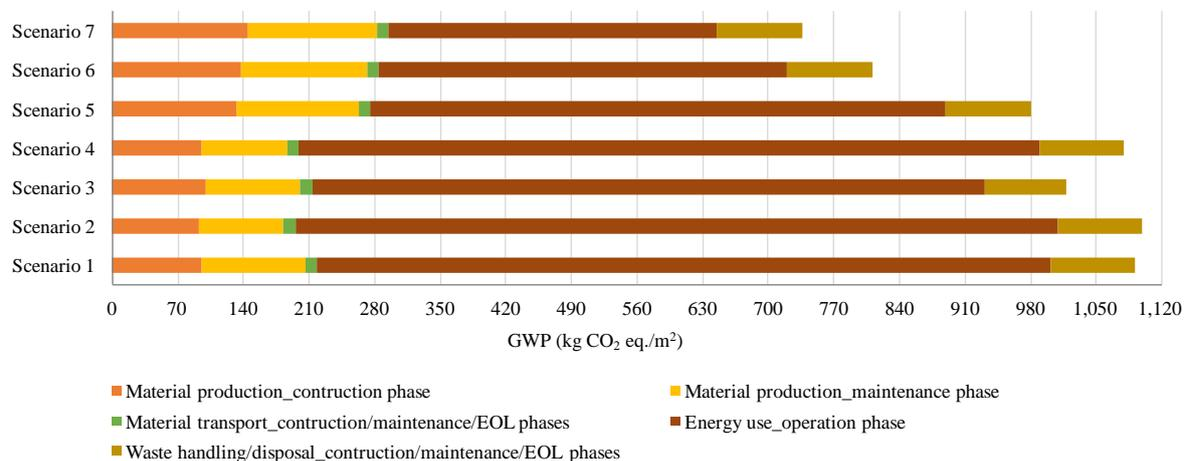
**Figure 3.** Global warming potential results normalized by the floor area and referred to 50 years of building life span after the renovation.
