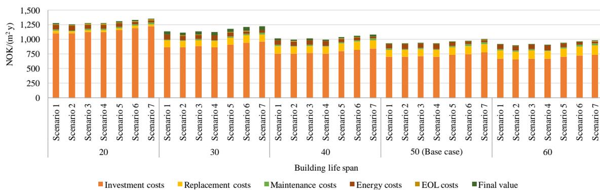
**Figure 9.** Equivalent annual cost results for different building life spans after renovation, normalized by the floor area.
