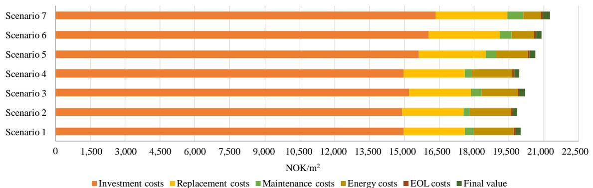
**Figure 5.** Net present cost results normalized by the floor area and referred to 50 years of building life span after the renovation.
