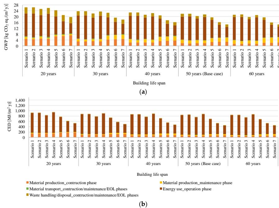
**Figure 7.** Results of global warming potential (a) and cumulative energy demand (b) for different building life spans after the renovation, normalized by the floor area and number of years.
