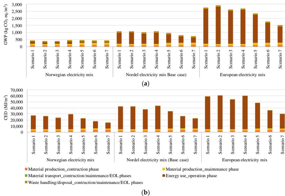
**Figure 8.** Results of global warming potential (a) and cumulative energy demand (b) for different electricity mixes, normalized by the floor area and referred to 50 years of building life span after the renovation.
