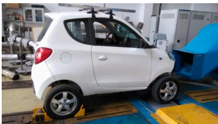
**Figure 11.** Road simulation test.
