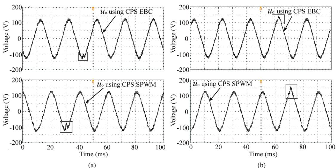
**Figure 17.** The experiment results of the five-level prototype under cases of load steps. (a) load steps as  $50 \Omega \rightarrow 25 \Omega$ ; and (b) load steps as  $25 \Omega \rightarrow 50 \Omega$ .
