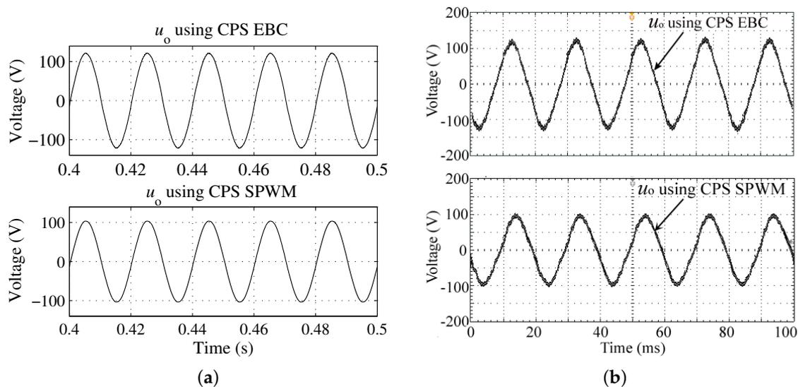
**Figure 11.** The results of the five-level prototype under the case of power imbalance ( $u_1 = 65$  V and  $u_2 = 80$  V). (a) Simulation results; and (b) Experimental results.
