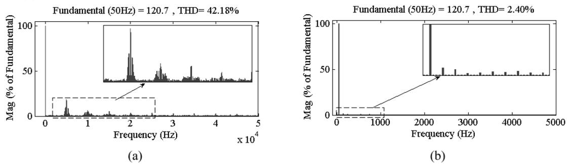
**Figure 10.** The FFT analysis result of the experimental prototype. (a) The stepped voltage  $u_{AB}$ ; and (b) The output voltage  $u_o$ .
