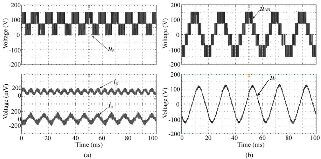
**Figure 9.** The experimental results of the operation of the five-level prototype using CPS EBC. (a) The output voltage  $u_g$  of the first stage (figure top); The current  $i_g$  and  $i_o$  (figure bottom); and (b) The stepped voltage  $u_{AB}$  (figure top); The output voltage  $u_o$  (figure bottom).
