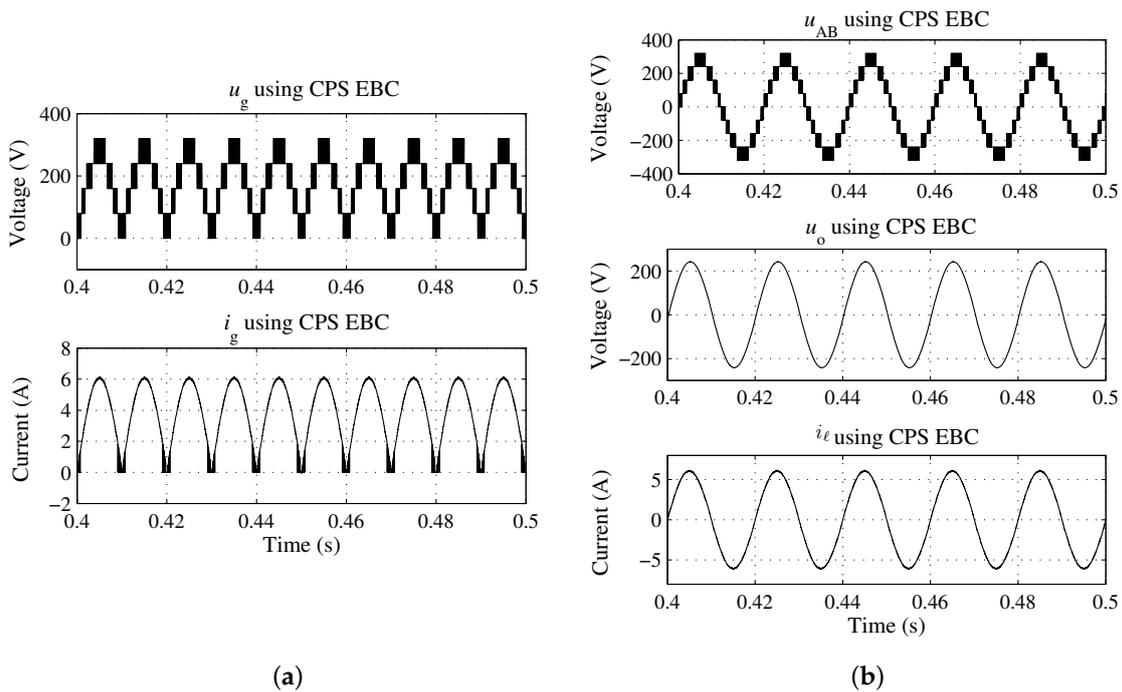
**Figure 8.** The simulation results of the nine-level prototype. (a) The output voltage  $u_g$  and current  $i_g$  of the first stage; and (b) The output voltage  $u_o$  and current  $i_o$  of the second stage.
