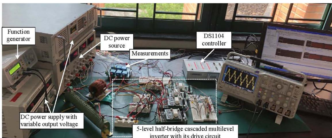
Figure 4. The hardware and interface of the experimental prototype.
