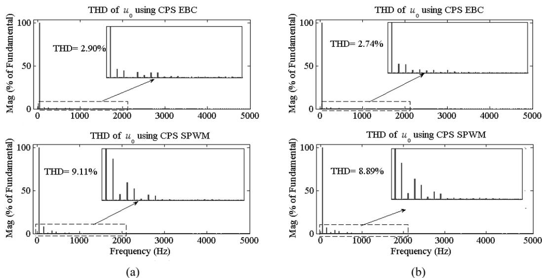
**Figure 15.** The comparison of the THD of the five-level experimental prototype under the case of DC voltages with fluctuations. (a) DC voltage  $u_1$  contains a ripple with a frequency of 100 Hz and an amplitude of 16 V; and (b) DC voltage of each cascaded unit contains a frequency of 100 Hz and an amplitude of 8 V.
