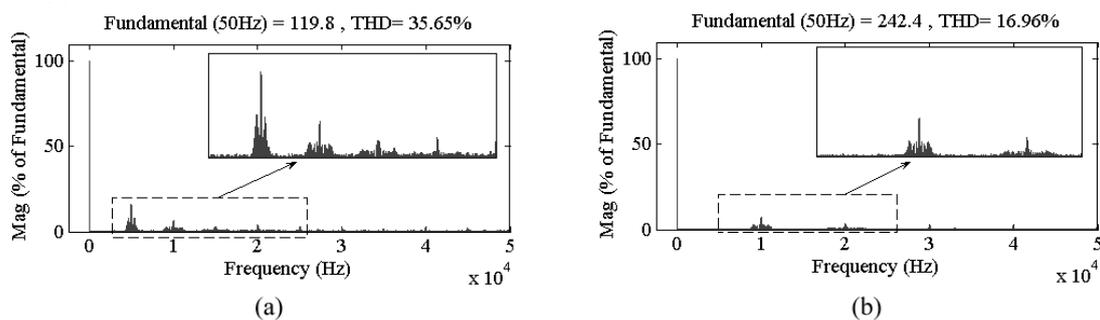
**Figure 7.** The fast fourier transform (FFT) analysis result of  $u_{AB}$ . (a) The five-level simulation prototype; and (b) The nine-level simulation prototype.
