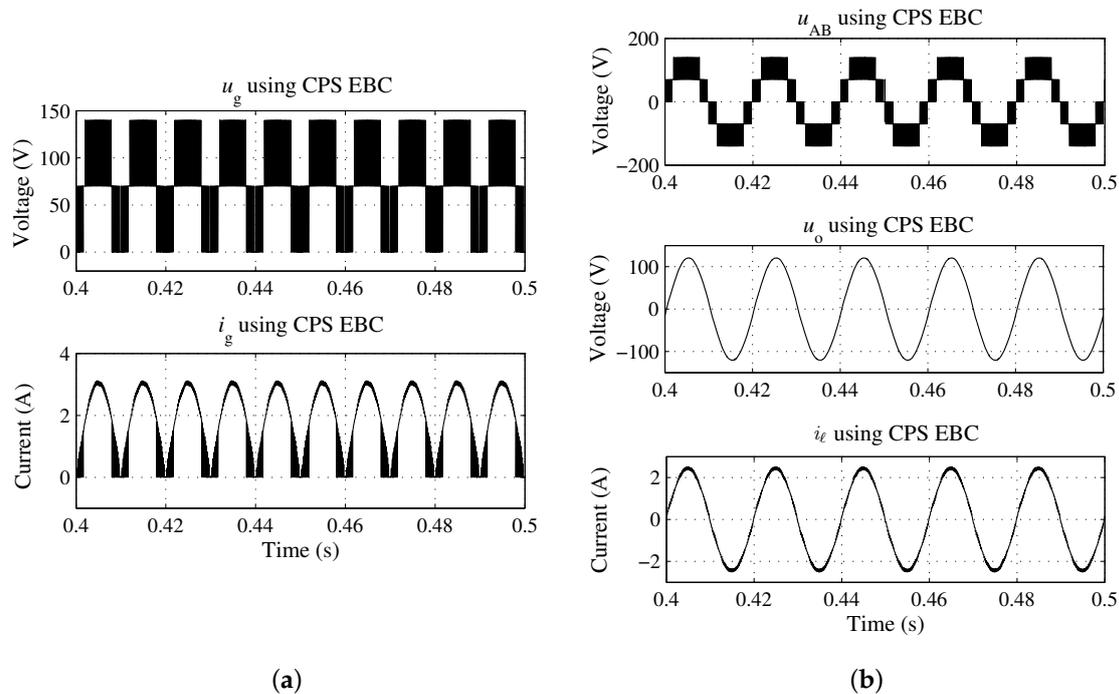
**Figure 6.** The simulation results of the five-level prototype. (a) The output voltage  $u_g$  and current  $i_g$  of the first stage; (b) The output voltage  $u_o$  and current  $i_o$  of the second stage.
