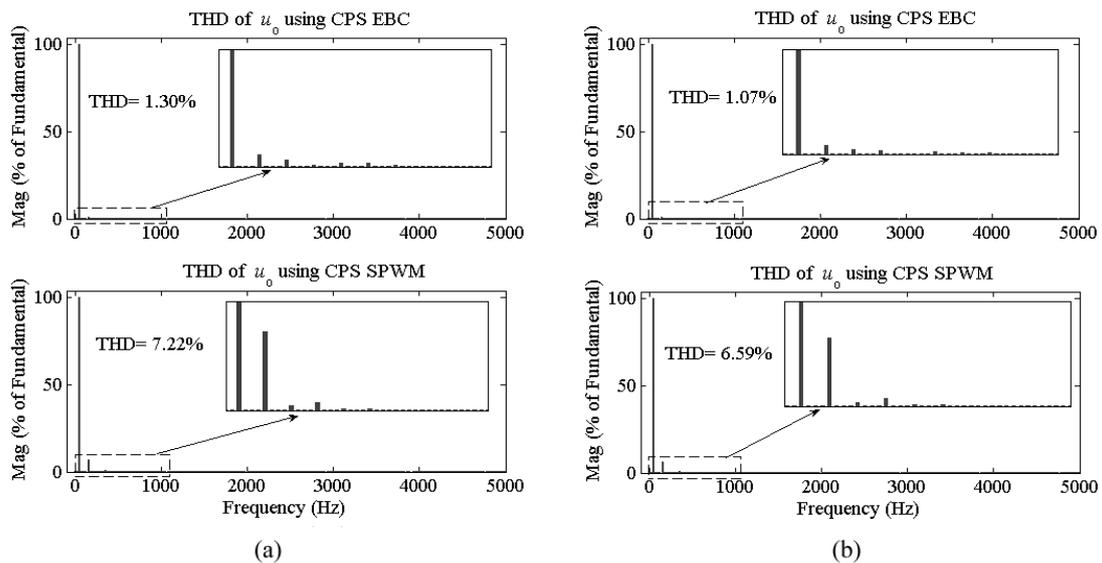
**Figure 13.** The comparison of the THD of the five-level simulation prototype under the case of DC voltages with fluctuations. (a) DC voltage  $u_1$  contains a ripple with a frequency of 100 Hz and an amplitude of 16 V; and (b) DC voltage of each cascaded unit contains a frequency of 100 Hz and an amplitude of 8 V.
