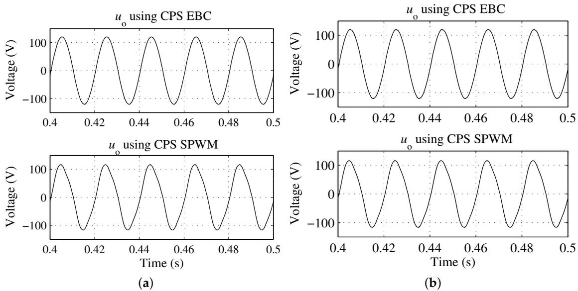
**Figure 12.** The simulation results of the five-level prototype under the case of unbalance DC voltages and DC voltages with fluctuations. (a) DC voltage  $u_1$  contains a ripple with a frequency of 100 Hz and an amplitude of 16 V; and (b) DC voltage of each cascaded unit contains a frequency of 100 Hz and an amplitude of 8 V.
