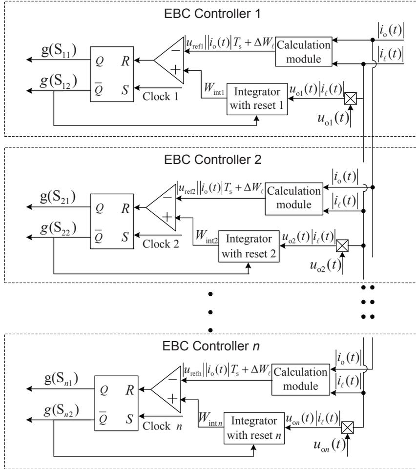
**Figure 3.** The structure of the CPS EBC method for the topology leaving out the details of the second stage.
