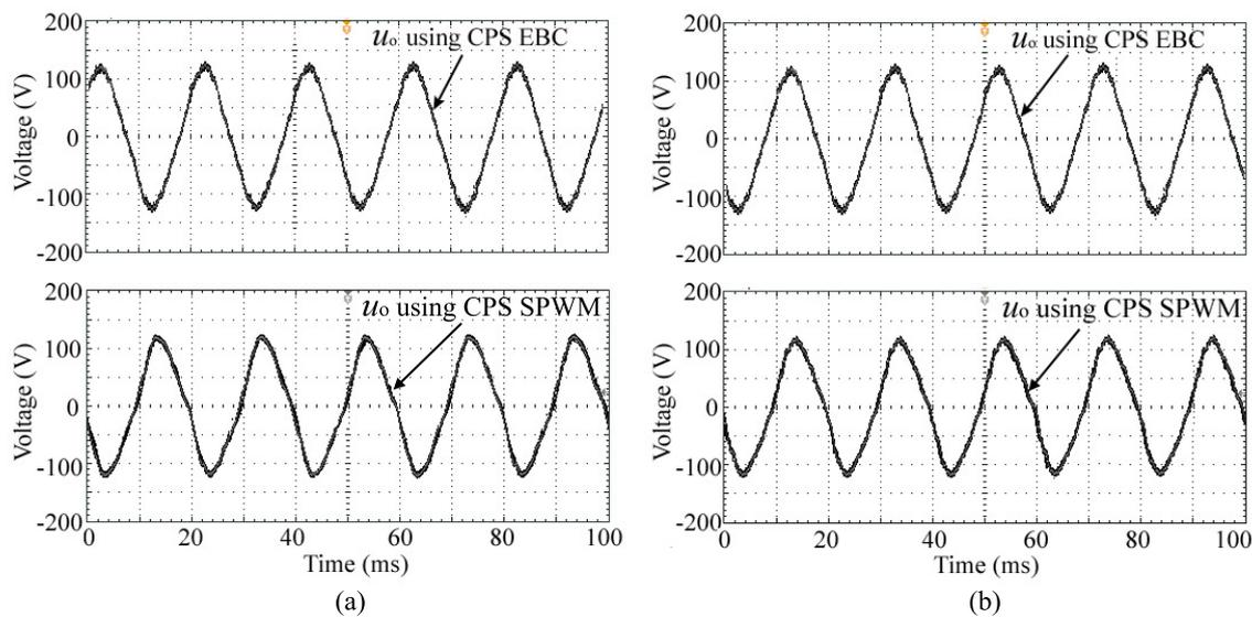
**Figure 14.** The experimental results of the five-level prototype under the case of DC voltages with fluctuations. (a) DC voltage  $u_1$  contains a ripple with a frequency of 100 Hz and an amplitude of 16 V; and (b) DC voltage of each cascaded unit contains a frequency of 100 Hz and an amplitude of 8 V.
