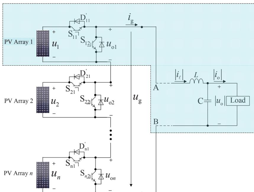
**Figure 2.** The structure of the topology leaving out the details of the second stage.
