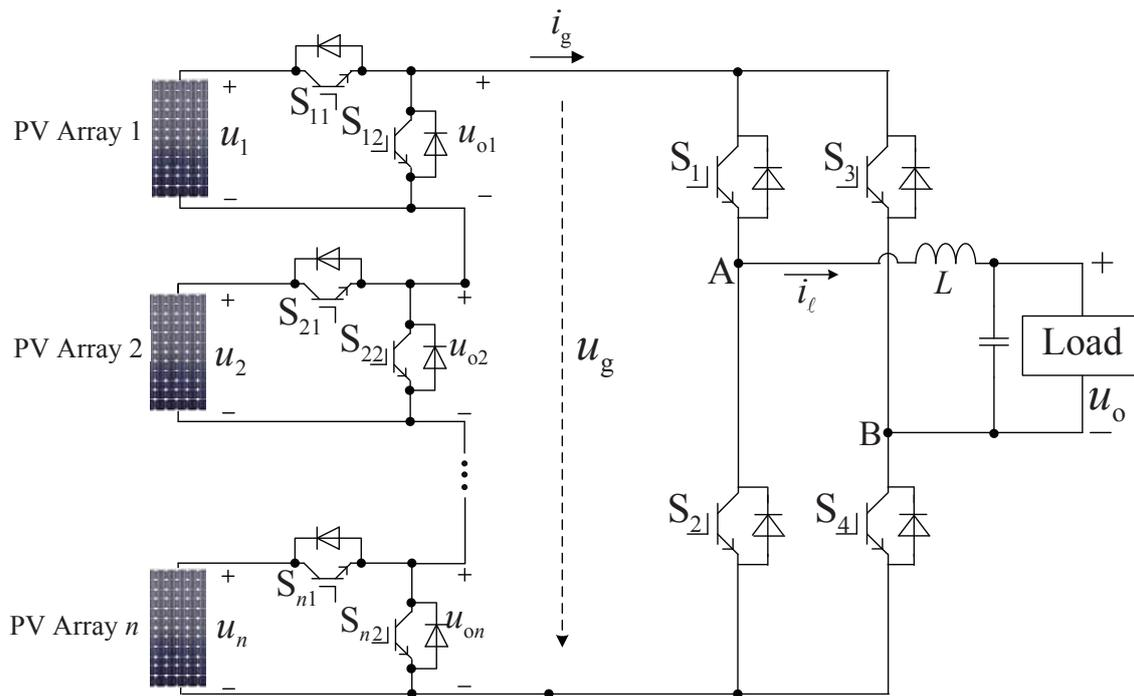
**Figure 1.** Standalone solar PV system with a cascaded half-bridge multilevel inverter.
