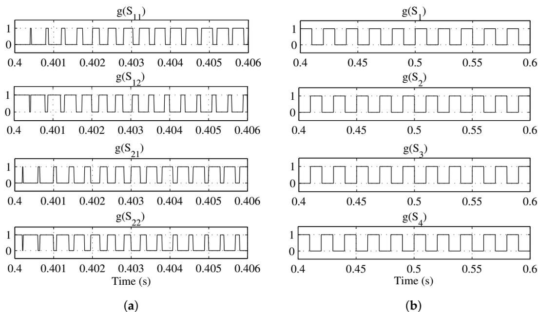
**Figure 5.** Gate signals of the five-level simulation prototype. (a) The gates of the first stage; and (b) The gates of the second stage.
