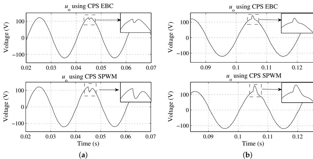
**Figure 16.** The simulation results of the five-level prototype under cases of load steps. (a) load steps as  $50 \Omega \rightarrow 25 \Omega$ ; and (b) load steps as  $25 \Omega \rightarrow 50 \Omega$ .
