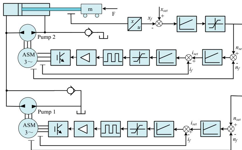
**Figure 8.** The principle to control differential cylinders with two speed variable pumps.
