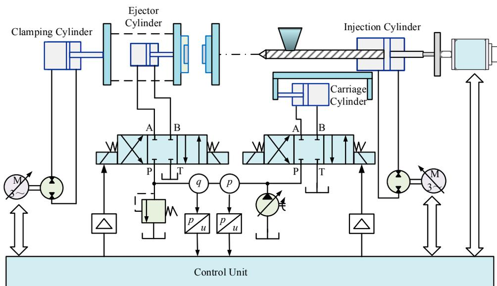
Figure 7. The hybrid control scheme of an electric-hydraulic IMM.
