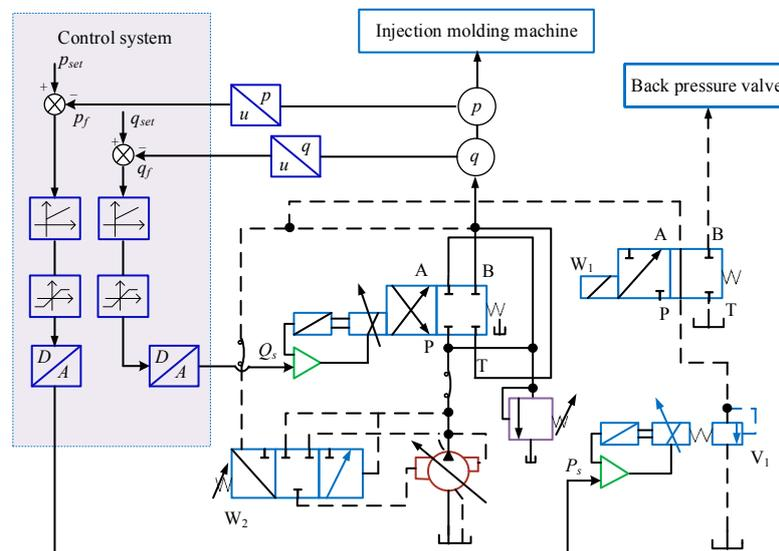
**Figure 5.** The schematic diagram of a load-sensing control system.
