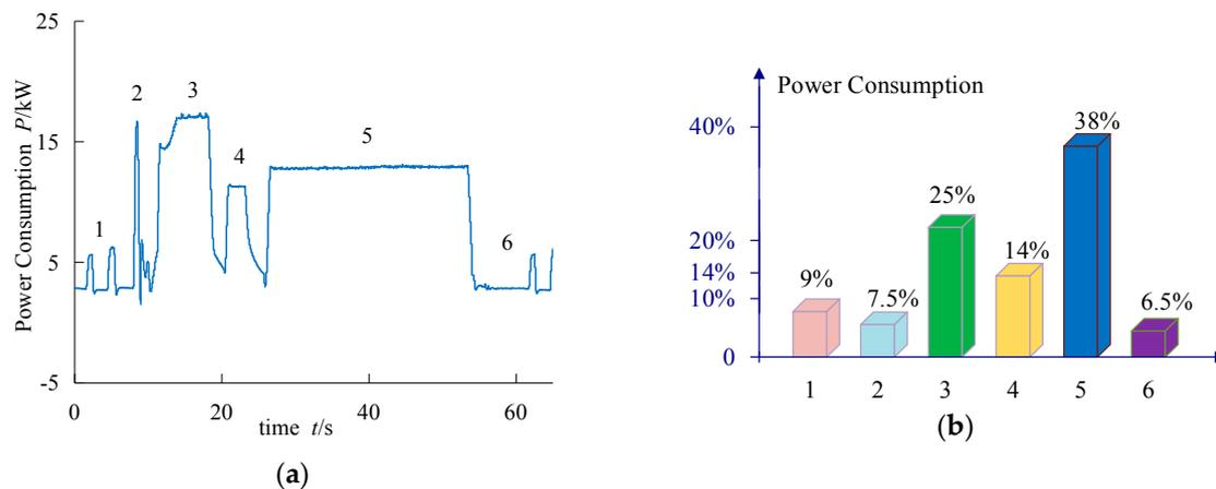
**Figure 3.** The distribution of power consumption of a hydraulic injection-molding machine (IMM) in a work cycle: (a) The power curve, (b) The distribution of power consumption
