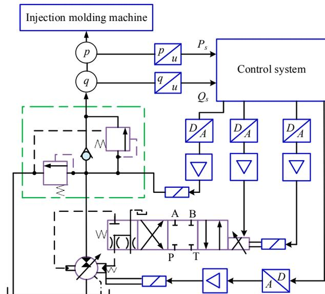
Figure 6. The electro-hydraulic system controlled P/Q compound proportional pump.
