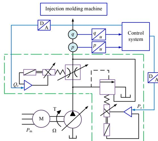
**Figure 4.** The structure diagram of a fixed displacement pump drive system.
