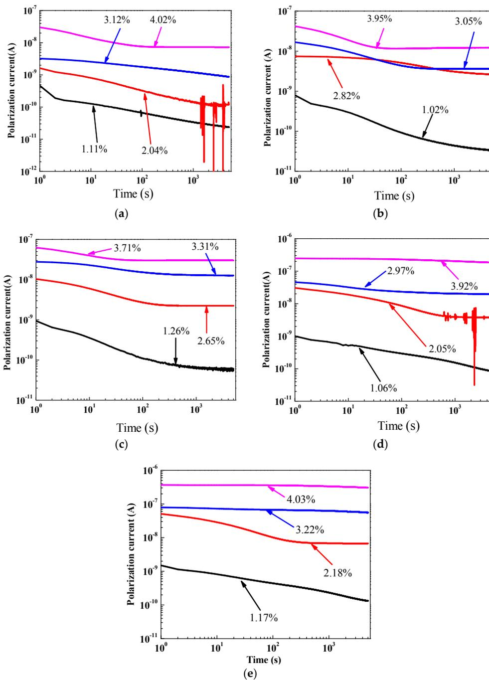
**Figure 1.** Polarization current results of oil-impregnated pressboards. (a) Aged 0 day; (b) Aged 8 days; (c) Aged 21 days; (d) Aged 32 days; and (e) Aged 42 days.
