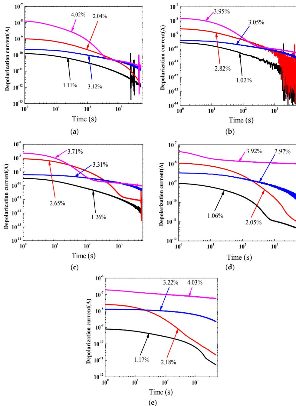
**Figure 2.** Depolarization current results of oil-impregnated pressboards. (a) Aged 0 day; (b) Aged 8 days; (c) Aged 21 days; (d) Aged 32 days; and (e) Aged 42 days.
