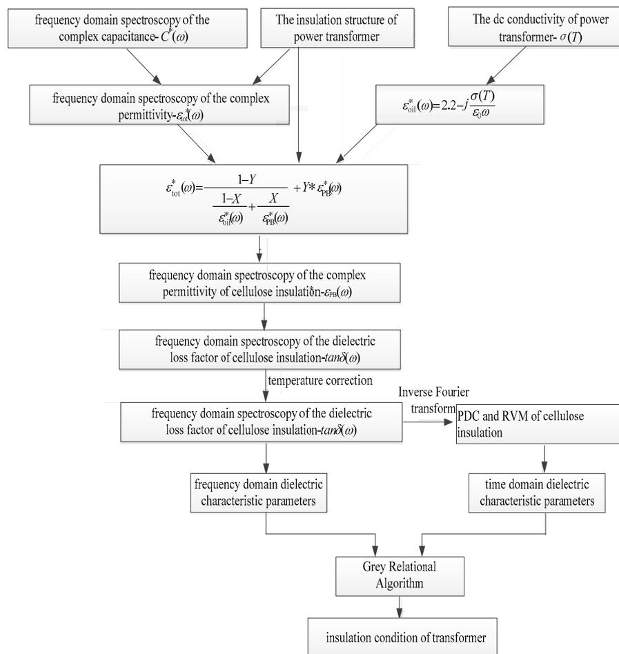
**Figure 6.** Flow chart of transformer insulation condition evaluation. PDC: polarization-depolarization current; RVM: recovery voltage measurement.
