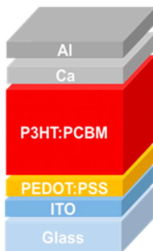
Figure 8. Sketch of the investigated polymer:fullerene solar cells. Sixteen devices have been fabricated and analyzed for each solvent-type.
