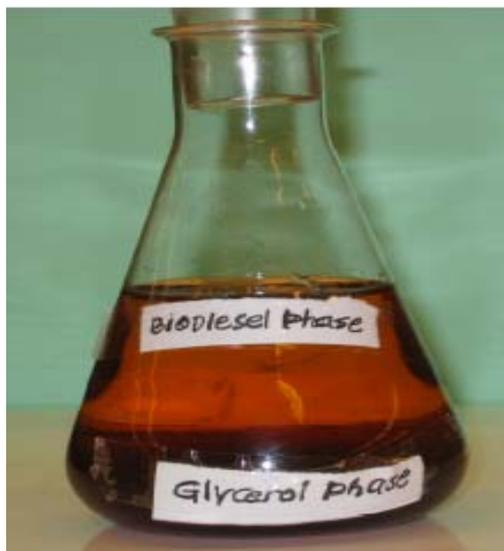
**Figure 8.** Biodiesel washing using distilled water.
