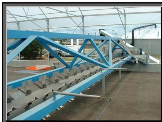
Sludge is, under current operating conditions, moved approximately 10 m along the drying beds each day; the average drying time is about 10 days. Once the biosolids material has reached the outlet end of the drying beds, it remains in a stockpile zone for an average of two days before being pushed by the turner mechanism onto a conveyor and loaded into trucks for transport from the site.
