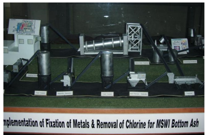
(b) Removal process model of heavy metals and chlorides from MSWI bottom ash.
