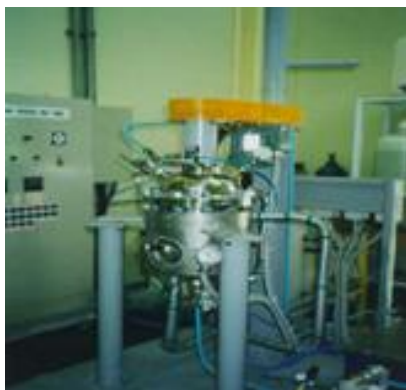
(b) Main reactor for PCC manufacture
