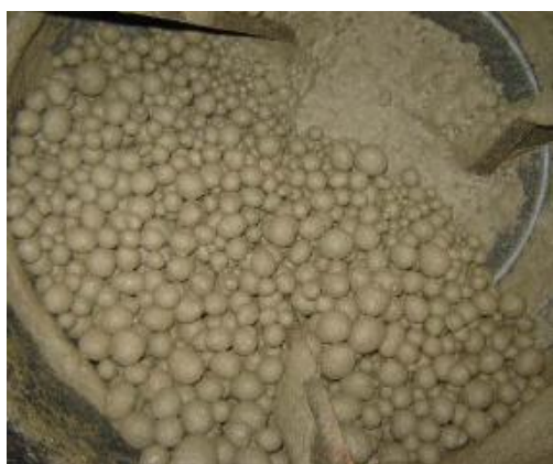
Figure 13. Artificial aggregate in mini concrete mixer (from Melton et al. [37] with permission of J.S. Melton).
