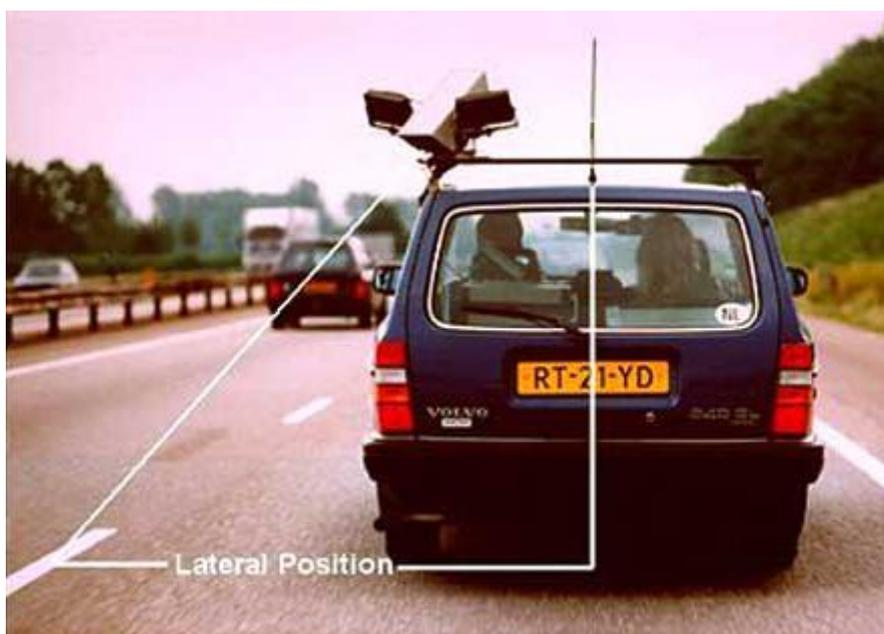
Note that the camera for lateral position measurements is equipped with two infrared lights, to enable recording during the night and dark weather circumstances. Adapted with permission from reference [12].
