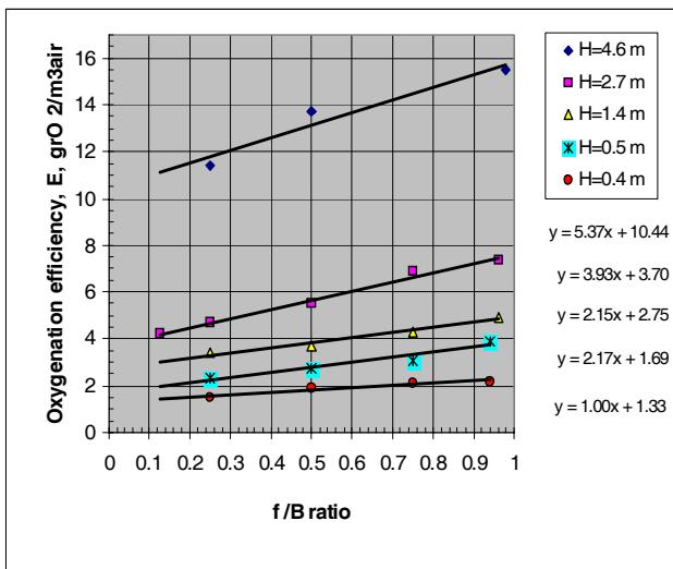
**Figure 8:** Effect of (f/B) ratio on oxygenation efficiency (E) of the system at constant air flow rate.
