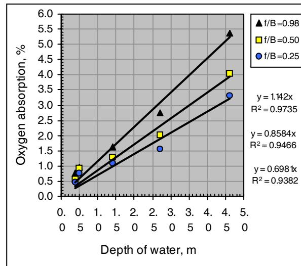
**Figure 9:** Effect level of depth of water (h) on oxygen absorption ( $\delta$ ) at constant air flow rate.
