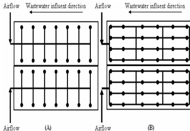
**Figure 3:** Two types of diffusers placement. (A): transverse arrangement. (B): longitudinal arrangement
