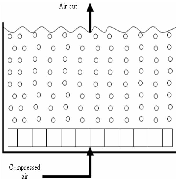
**Figure 1:** Schematic of diffused air aeration system
