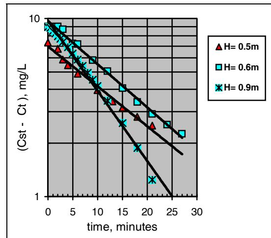
**Figure 4:** Sample of the experimental results showing the variation of  $\log(C_{st} - C_t)$ , mg/L over time at various water depths.
