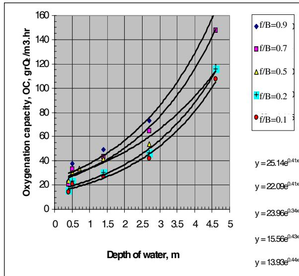
**Figure 5:** Effect of depth of water on the oxygen transfer capacity (OC) of the system air at constant air flow rate.
