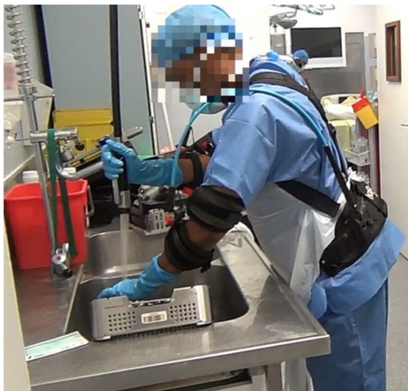
Figure 2. Healthcare worker wearing the exoskeleton during the task of cleaning surgical tools.
