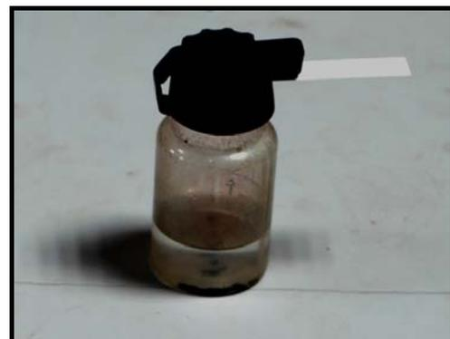
**Figure 1:** Experimental set up for strip test method used for detection of arsenic.
