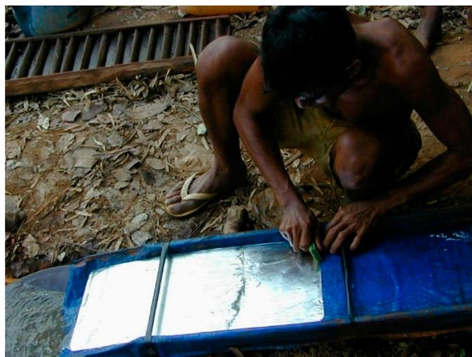
**Figure 5.** Scraping mercury with gold from flume. (T. Murphy).
