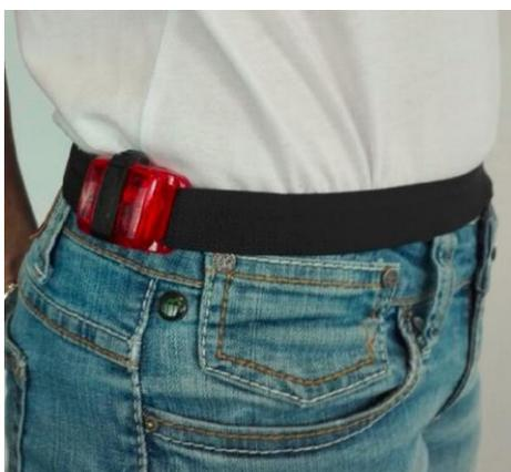
**Figure 2.** Students wore the ActiGraph GT3X-BT on the right hip attached with an elastic belt.
