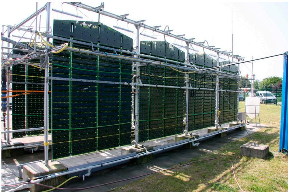
Figure 6. Flat panel photobioreactors (PBRs) cultivation system.
