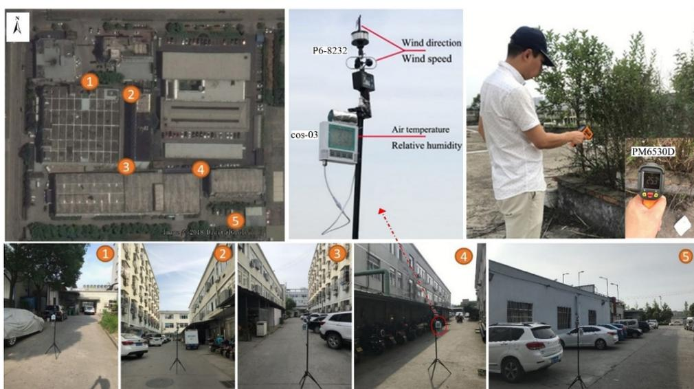
Figure 5. On-site field measurement and the spatial distribution of test points.
