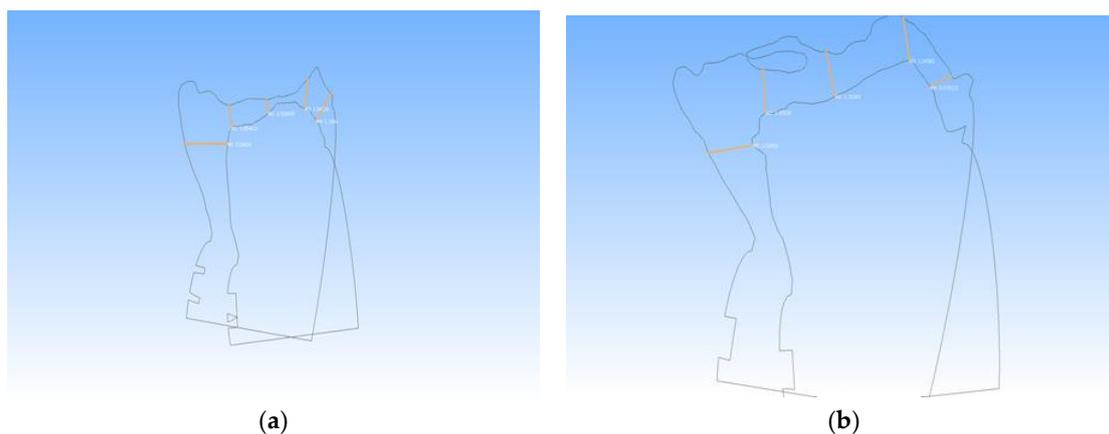
**Figure 6.** Measuring the line spacing between the two outer contours of the models in different slices. (slice  $-1.5$  and  $2.5$ ). (a) slice  $1.5$  mm and (b) slice  $2.5$  mm.
