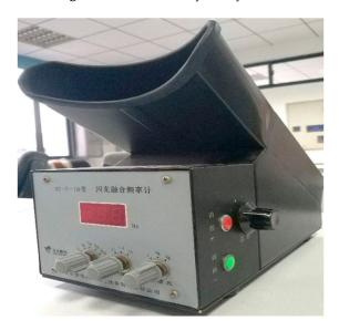
Figure 4. EP403 highlight scintillometer.
