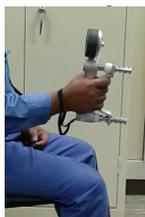
**Figure 1.** Measurement of the grip hand force using the JAMAR dynamometer with the second handle position (span = 45 mm).
