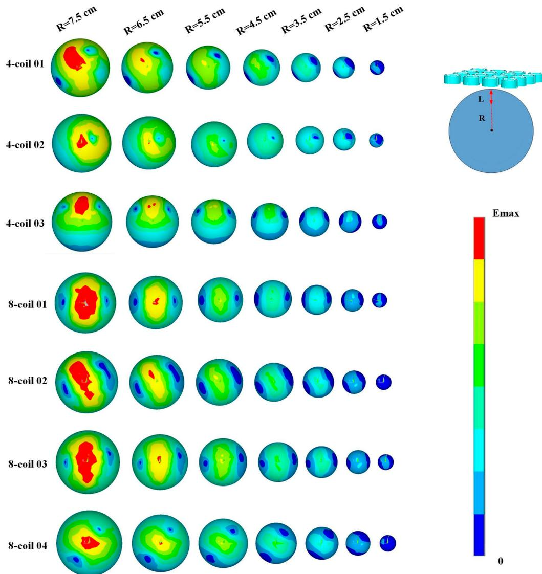
**Figure 8.** Spatial distribution of the induced EF in different layers of the head model. R meets the relationship of “ $R = 8.5 \cdot L$ ”, indicating that R attenuates with the increase of L.
