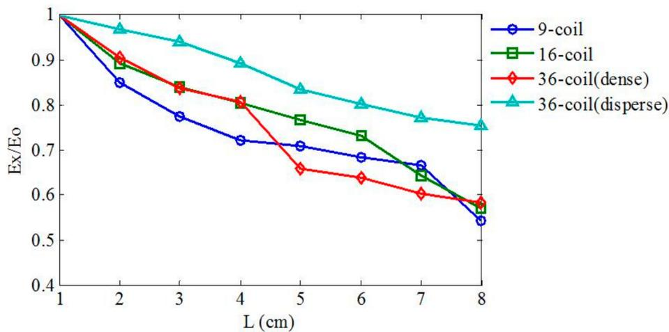
**Figure 6.** The variation tendency of EF intensity generated by multi-coil arrays of distinct dimensions. The size of an individual coil and an overall spatial distribution of arrays are both influential factors to the variation tendency of the induced EF.
