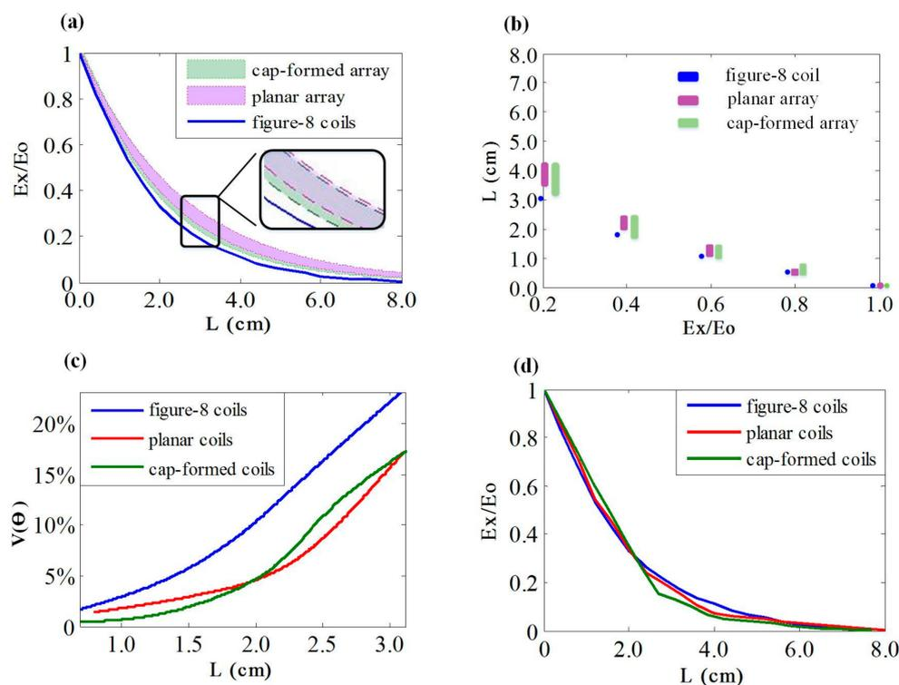
**Figure 12.** (a) Attenuation rate of induced EF in the figure-8 coil, the 36-coil planar array, and the 36-coil cap-formed array. (b) Corresponding ranges of activated depth with different coil types. (c) The focality of various coils with optimal energizing strategies. (d) The attenuation rates of the figure-8 coil, the planar array, and the cap-formed array with optimal energizing strategies.
