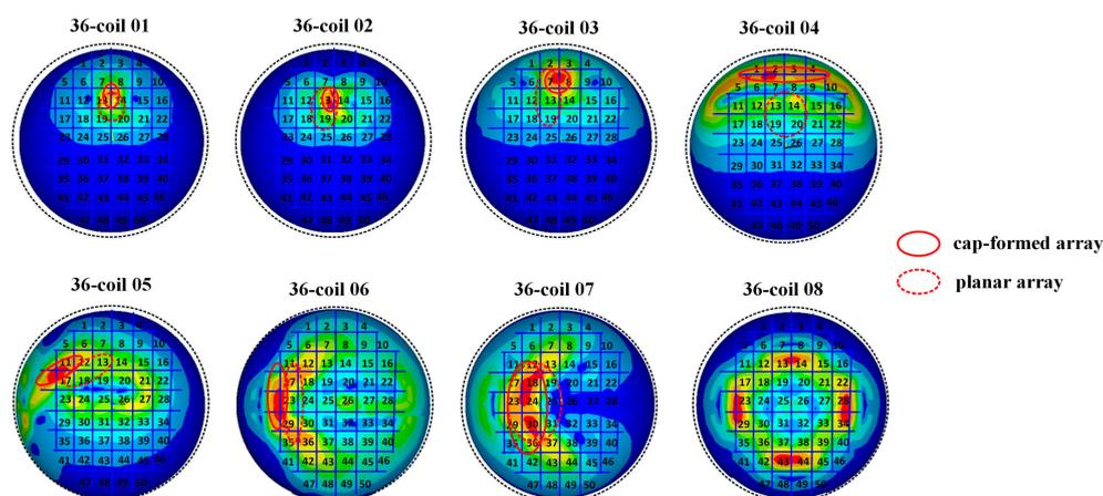
**Figure 13.** The comparison of the planar array and the cap-formed array. Red full lines indicate cortical regions activated by the selected coils in the cap-formed array. The dashed lines show cortical tissues stimulated by the same corresponding coils in the planar array.
