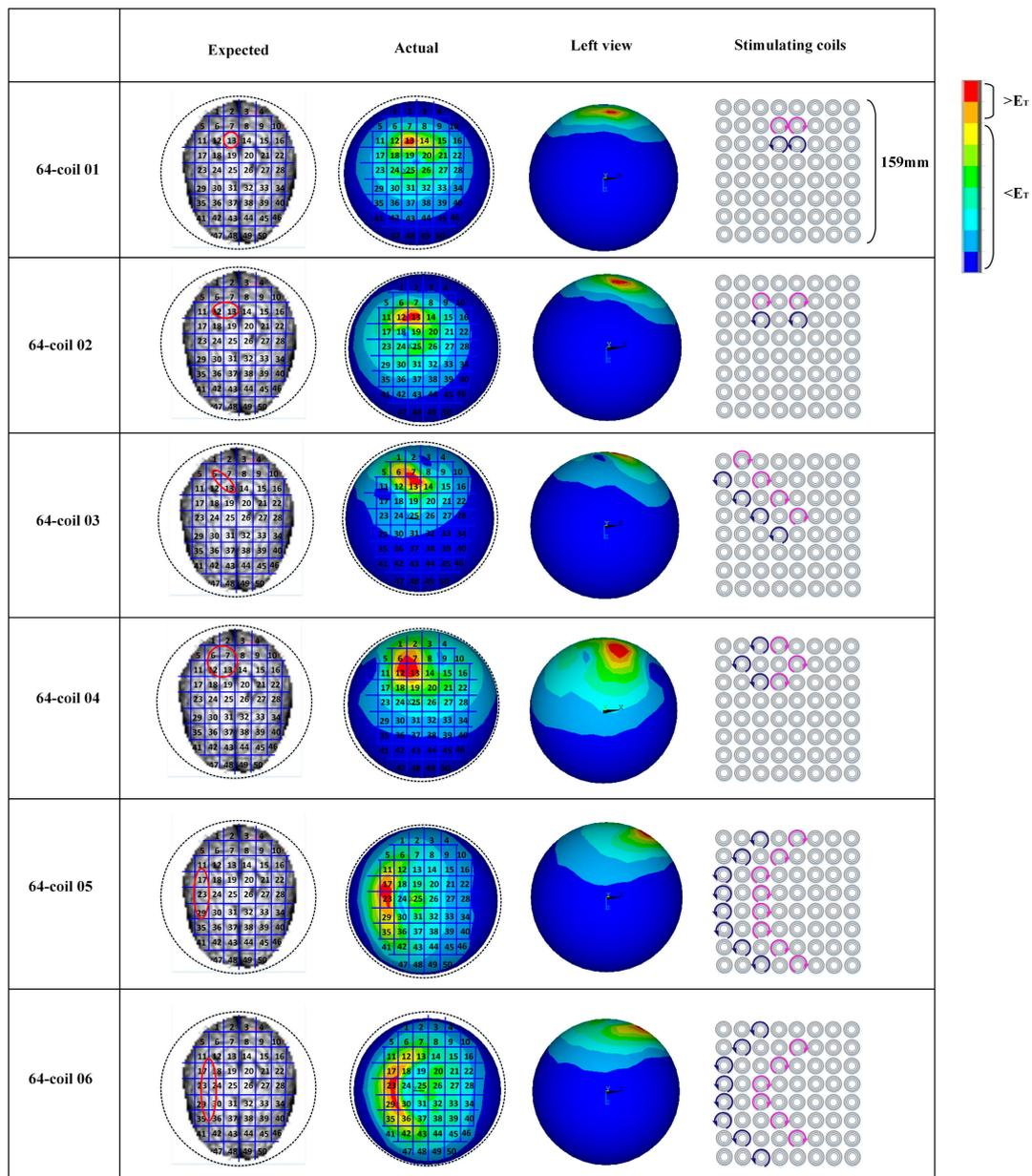
**Figure 11.** Stimulation results targeted at different cortical tissues. The units in red solid circles are interested regions. The activated parts and energized coils are shown correspondingly. Here, currents in coils are indicated by arrows of different directions.
