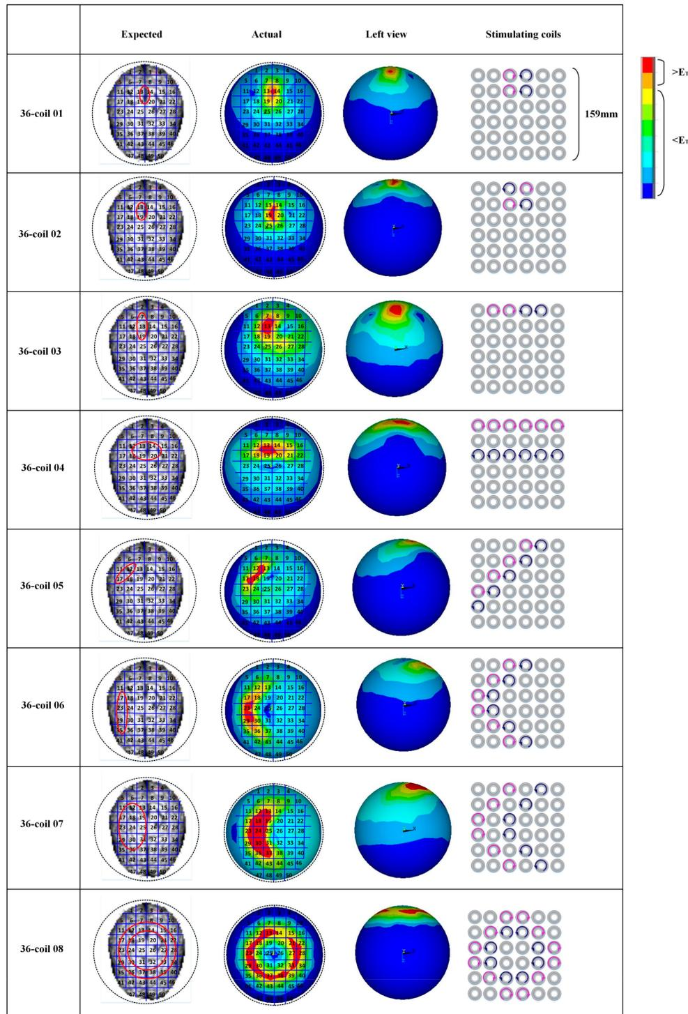
**Figure 10.** Stimulation results targeted at different cortical tissues. The units in red solid circles are interested regions. The activated parts and energized coils are shown correspondingly. Here, currents in coils are indicated by arrows.
