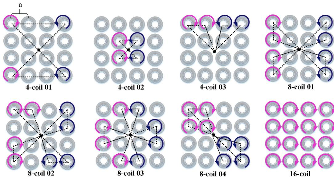
**Figure 4.** Sketch maps of different coil combinations based on the 16-coil array. Current directions are indicated by arrows. Coils with clockwise or anticlockwise current are regarded as stimulating coils, whereas the gray ones represent coils without electricity. “a” indicates the length between two adjacent coils and the connecting lines in each coil array mark out the specific areas corresponding to different energized coil combinations.
