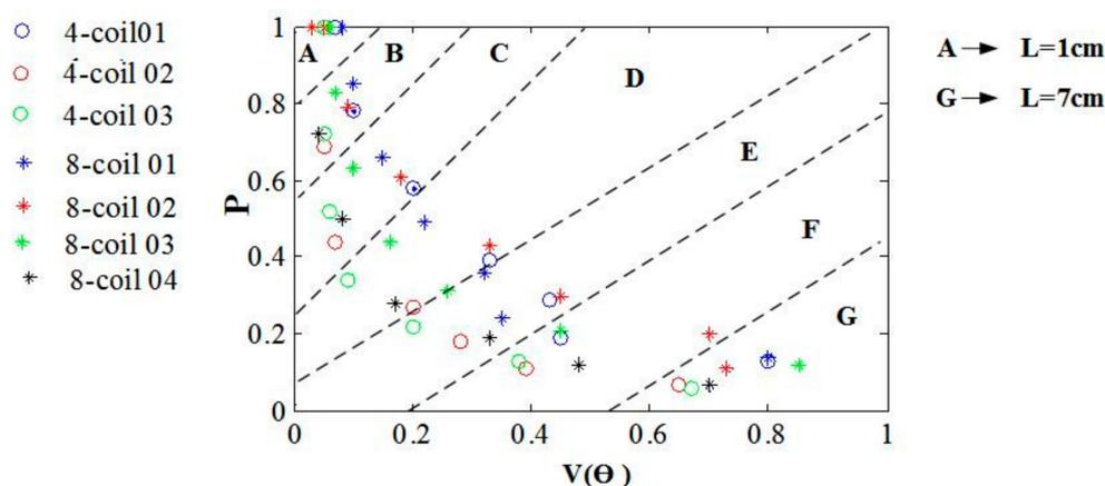
**Figure 9.** Strengths of the induced EFs at different depth are normalized with respect to the maximum EF amplitude estimated on the cortex. The values of proportion are represented with P.  $V(\theta)$  shows the activated volume of the head model. The depths of brain tissue are marked A–G, which correspond to L from 1 to 7 cm.
