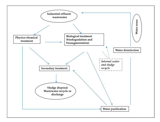
Figure 1. Generic flow of industrial wastewater treatment plan (adapted and modified from [4]).
