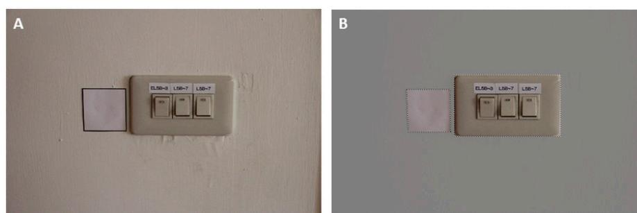
**Figure 1.** Raw (A) and processed photographs (B) that were used to determine the surface area of a light switch. The number of pixels in the reference paper (5 × 5 cm) and the surface of interest were calculated using the processed photographs. The equation used to calculate the surface area is described in the Methods Section.
