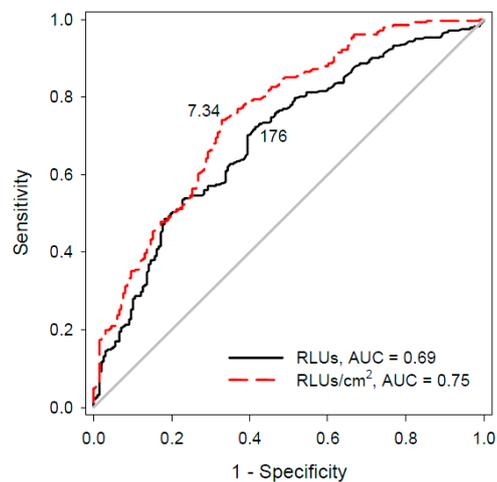
**Figure 3.** Receiver-operating characteristic (ROC) curves of the criteria based on the non-adjusted ATP-based values (RLU; solid black line) and adjusted ATP-based levels (RLU/cm<sup>2</sup>; dashed red line) versus the microbial growth-based values. Culture-based levels of >2.5 CFU/cm<sup>2</sup> were regarded as culture positive. The best cut-off points demonstrated by both curves were determined using the Youden index. AUC refers to the area under the curve.
