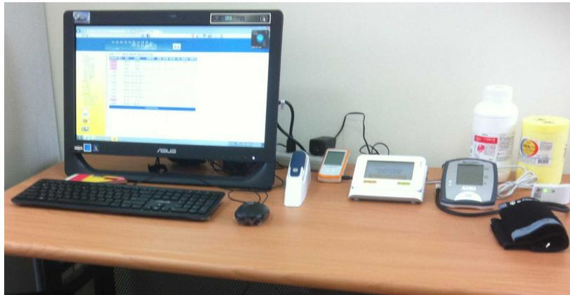
The hardware includes weight scale, blood pressure cuff, blood glucose meter, and pulse oximeter. The equipment measures vital signs tailored to residents' clinical needs, such as weight, blood pressure, blood glucose, heart rate, and oxygen saturation.
