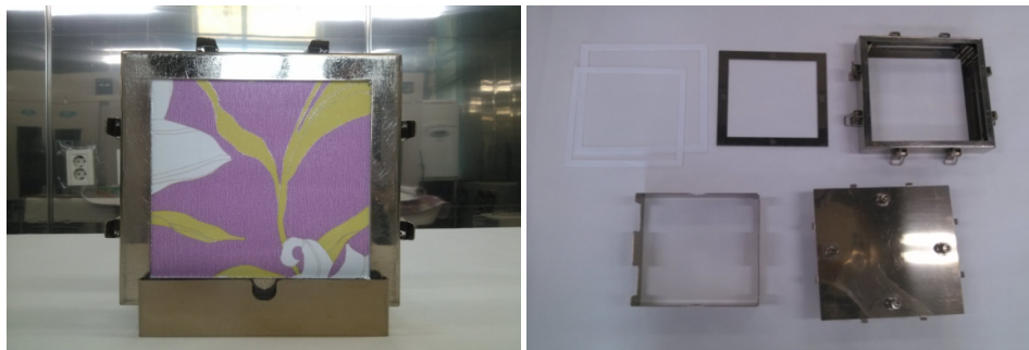
Figure 1. Photograph of an example wallpaper test sample. Parts of specimen holder Installed sample.
