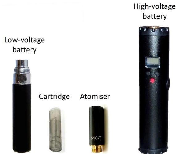
Both EC devices were tested on 4 s puffs [12]. It was found that the dry-puff phenomenon was consistently reproduced with the high-voltage device at 4 and 3 s puff duration. Therefore 2.5 s puffs were used with the high-voltage device, while 4 s puffs were used with the regular-voltage device.
