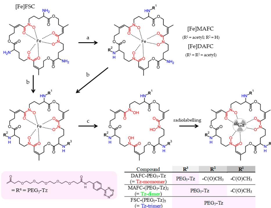
**Scheme 1.** Synthetic strategy for FSC-based tetrazine (Tz) conjugates [a: methanol and acetic anhydride (MetOH/Ac<sub>2</sub>O); b: Tz-PEG<sub>5</sub>-NHS/DMF/DIPEA; c: EDTA] radiolabelled with gallium-68.
