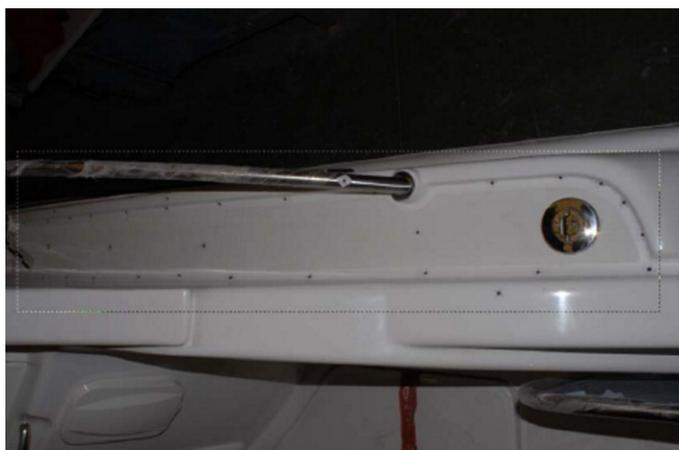
In order to scale the photogrammetric model, scale bars whose dimensions are known are located in the zone that is being measured. The bars have different sizes, and their total length varies between 30 and 50 cm. These dimensions allow them to be placed into a case with the rest of the equipment.
