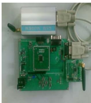
The GPRS modem (on the top) is connected to the motherboard through the serial line. The CC2430 module is inserted at the right corner of the motherboard, and the MSP430 minimum system board is in the middle of the motherboard.
