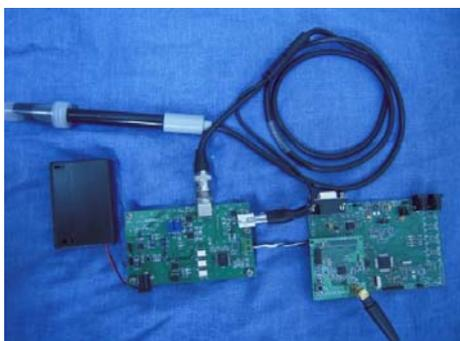
Its temperature measurement range is 0–80 °C, and the accuracy is  $\pm 0.5$  °C; its pH measurement range is 0–14, and the accuracy is  $\pm 0.05$ . The actual data base station is shown in Figure 22.
