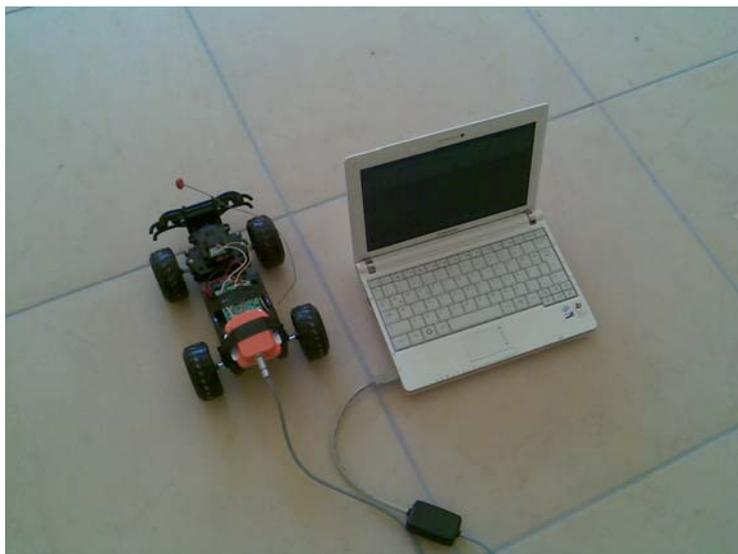
The experimental platform is shown in Figure 4. The Xsens IMU is attached to the body of the mobile vehicle and connected to the notebook PC with USB cable.
