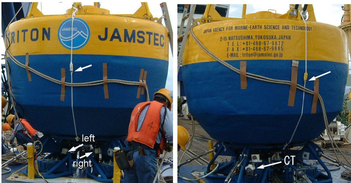
In addition to the regular CT sensor, we installed four small thermometers on the hull of a buoy that was deployed at 0°N, 156°E for about one year beginning in February 2005 (one thermometer stopped
