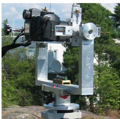
Figure 1. In order to create a measurable panoramic image, a concentric image acquisition was ensured with a calibrated camera mount.
