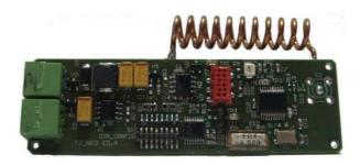
Finally an adapted antenna has been added. We have chosen a pig tail antenna (see Figure 5) which allows the design of the board to be thinner than by using a standard monopole. Because future experiment expectations will involve mammals, we wanted the secondary node to be as least uncomfortable as possible for the animals, without reducing range transmission capabilities. As shown in Figure 5, both the harvesting and transmission modules are located in the same board.
