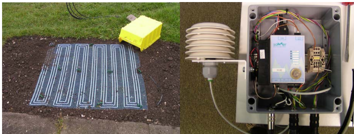
Figure 5. (left) Sensor mat for SOG detection. (right) IA in weather-proof box with an attached dew-point sensor.
