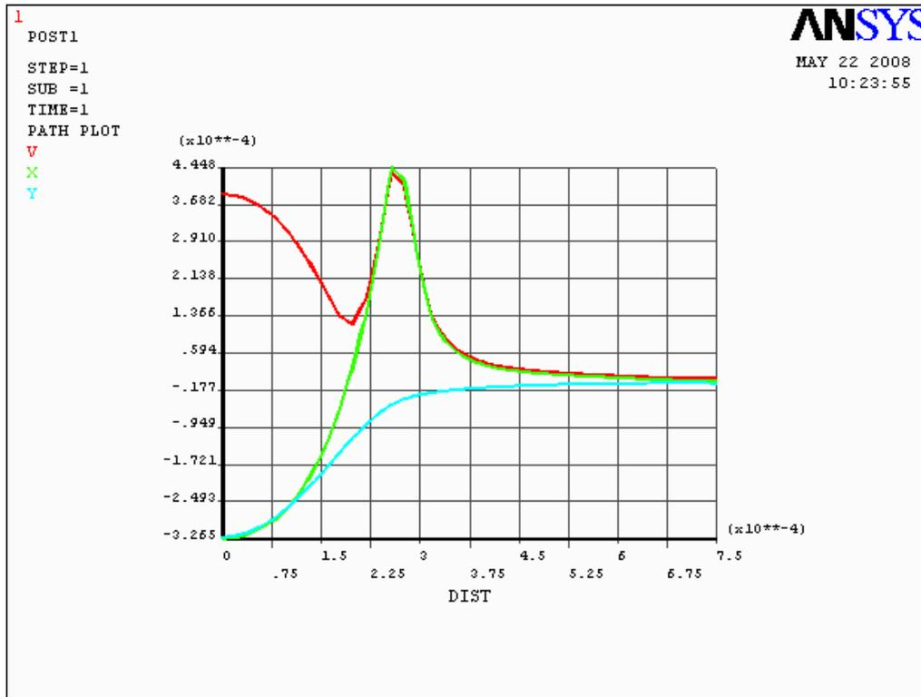
For a diaphragm size of  $520 \mu\text{m}$  by  $520 \mu\text{m}$  with a  $30 \mu\text{m}$  diaphragm thickness, comparison between the theoretical formula of the diaphragm and the ANSYS result shows that the simulation result agreed very well with the approximate solutions of Westergaard and Guckel, respectively [16]. Accordingly, we may conclude that ANSYS is an efficient method for calculation of the design for the given size of a diaphragm.
