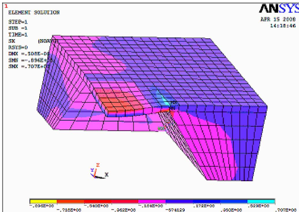
The quarter finite element models of the pressure sensors were established since a pressure sensor device with C type structure for a solid model has a quartered symmetry. The x-direction stress distribution is shown in Figure 1. The zone of stress concentration is located at the edge of the membrane, where the resistors are implanted.
