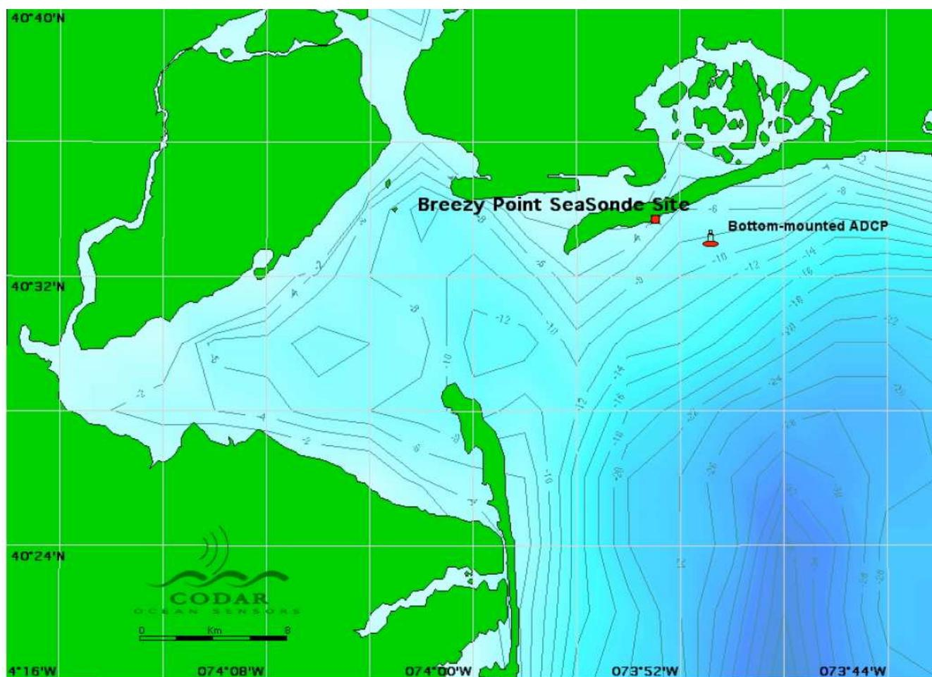
In our analysis, depth contours near the radar are assumed to be parallel to shore and the depth profile is obtained from Figure 12.
