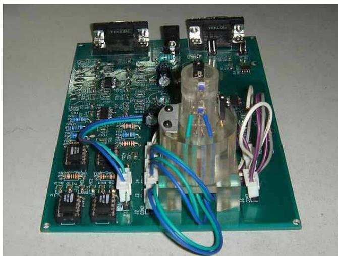
The structure of the detecting head in the photo is shown in Fig.6. The degree of blood oxygen saturation is measured through an independent module.
