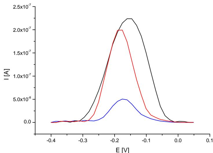
In reference examination with the use of DNA isolated from non-GM soybean MB signal was relatively high ( $0.191 \mu\text{A}$  at the peak potential of  $-0.176 \text{ V}$ ). The increase could have been explained by the failure of hybridization reaction and removing unbound soybean DNA from the electrode surface.
