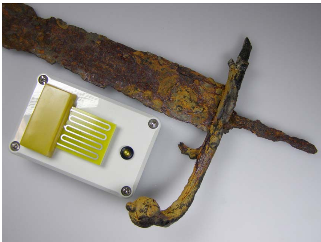
Figure 3. The CORRLOG sensor for monitoring corrosion in metallic artefacts. (Photo: courtesy of Tomas Prosek).
