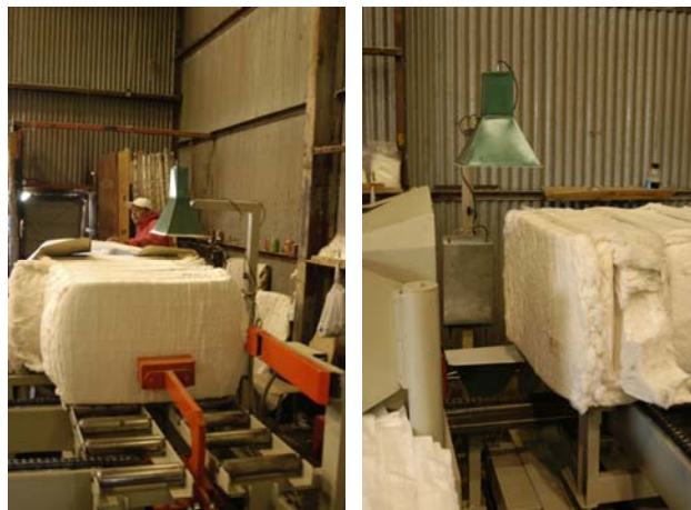
Figure 7. Shows how a bale is typically conveyed past the sensing station of one of the original prototype microwave moisture systems of the authors.
