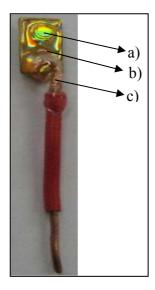
The developed electrode was secured on an adequate support provided with an electrical cable (contact pin MP3-type from Metrohm) which connects the electrode to the potentiostat.
