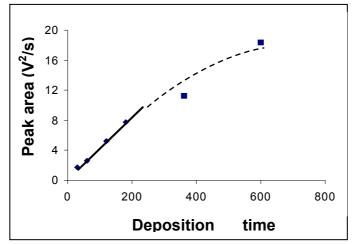
Although determination sensitivity increased with mercury deposition time, a value of 180 s for the deposition time was used in order to do not increase too much the durations of the analysis.
