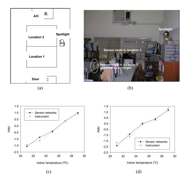
Two different algorithms, extrapolation and maximum entropy methods, were employed to estimate the data loss. Figure 6(c) and (d) show the PMV indices distribution in space that were obtained by the sensor networks with the extrapolated estimation and the maximum entropy method, respectively. It is
